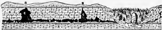
FIG. 38.—Diagram showing action of soil water in excavating caverns. A A , layers of limestone easily dissolved in soil water; B B , sink holes by which soil water enters the cave; C C , vertical shafts or domes; D D , horizontal galleries. At the right is a natural bridge, or remnant of a large cave.—After SHALER.
